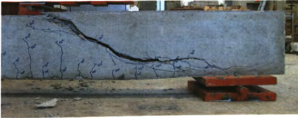
Figure 6.44. Control-NS-2 Beam at Failure
