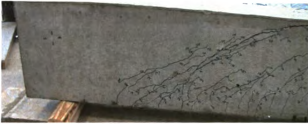
Figure 6.55. SCC-7-1 Beam at Failure
