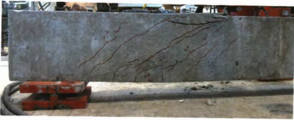
Figure 6.46. Control-7-1 Beam at Failure
