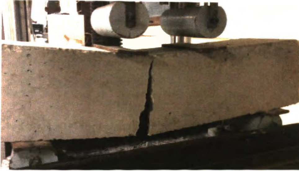
Figure 4.10. Modulus of Rupture After Testing
