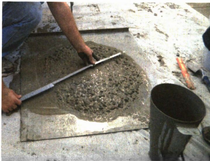
Figure 4.2. Measure Concrete Diameter During Slump Flow Test
