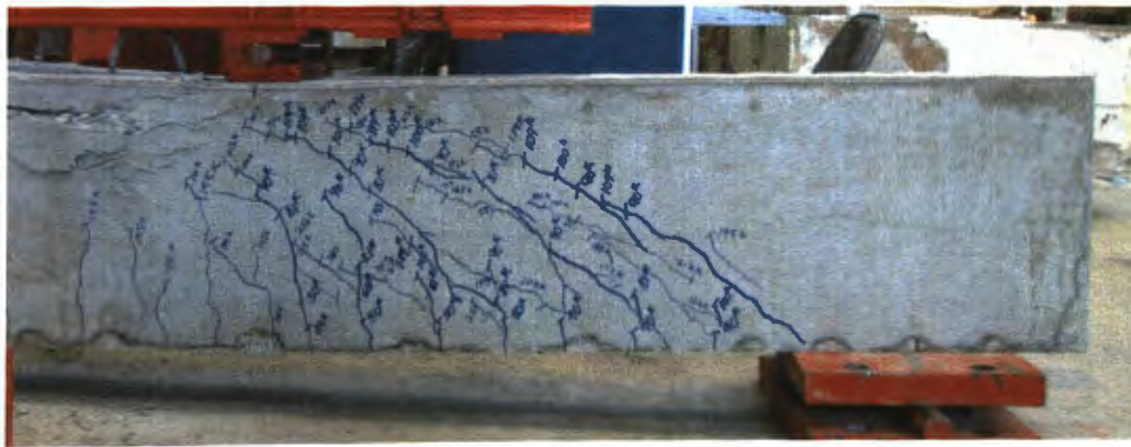
Figure 6.50. Control-5-2 Beam at Failure
